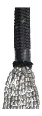
Braided rope manufactured with high tenacity polyester and an inside of several lead rosaries, that provide high density and low diameter to the lead line. Due to this construction, this rope has a great power of sinking, and thanks to its braided double cover of high tenacity polyester, it owns an excellent abrasion resistance.
